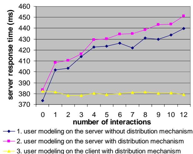
Figure 4: Performance Measurements
