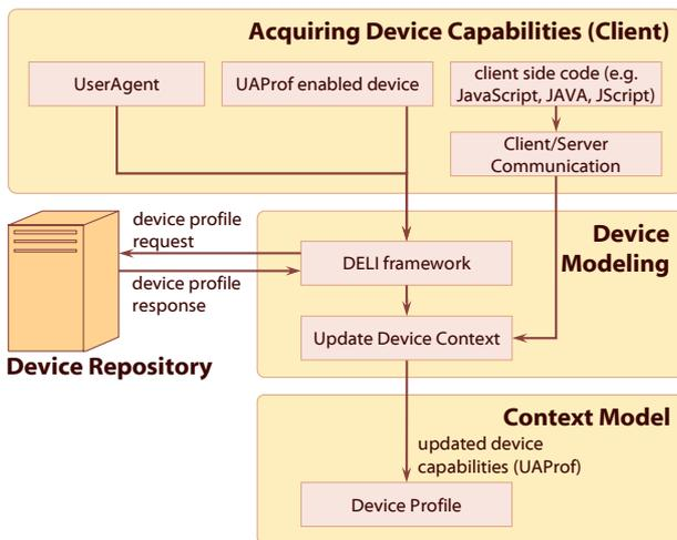
Figure 3: Modeling Device Capabilities
